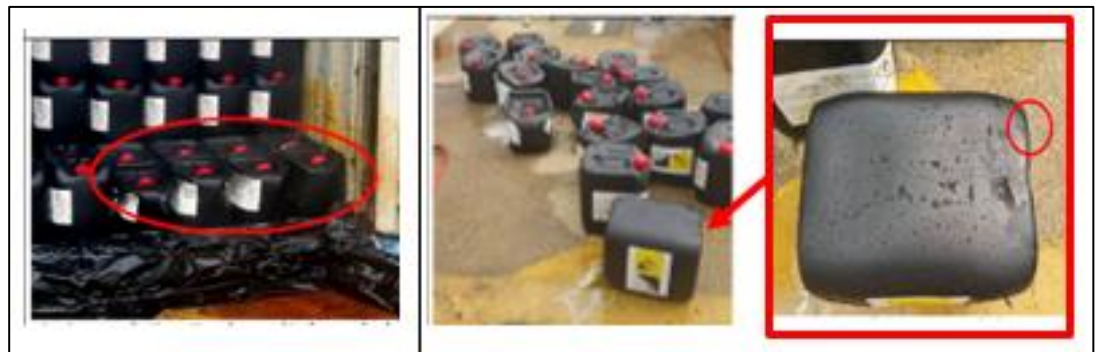
Figure 41 - Case 3, lower tier jerrican crushed and damaged (1 cm crack at the bottom of the jerrican) - Source: Regulator of the Port of Singapore
