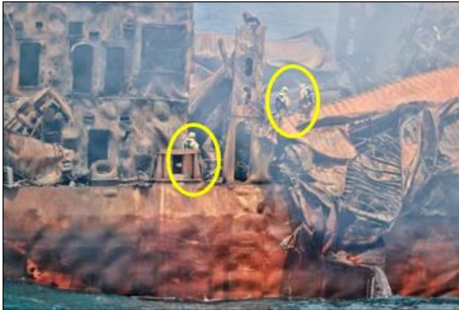
Figure 17 - Salvors onboard XP to inspect the extent of damage - Source: SLPA (annotation by TSIB)
