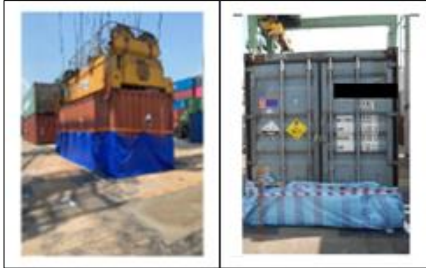
Figure 42 - Use of tarpaulin to minimise the spread of the leak - Source: Regulator of the Port of Singapore
