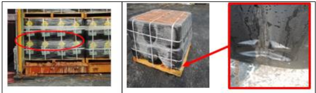
Figure 40 - Case 2, lower tier jerrican crushed and damaged (hairline crack at the bottom of the jerrican) - Source: Regulator of the Port of Singapore
