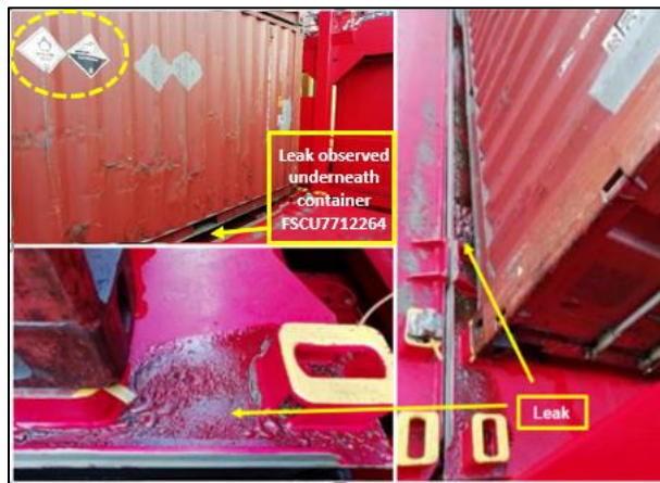
Figure 3 - Indicating leaked cargo observed underneath container and labelling of Primary (Corrosive) with Subsidiary risk (Oxidising agent) - Source: The Company (annotations by TSIB)
