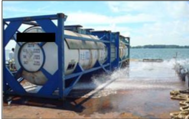
Figure 44 - Leaked ISO tank off-loaded onto a barge - Source: Regulator of the Port of Singapore
