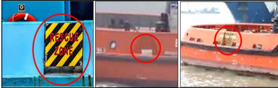
Figure 7: Examples of bulwark hinged doors on some tugboats (of a similar size). Some tugboats demarcated this access area as the rescue zone.
