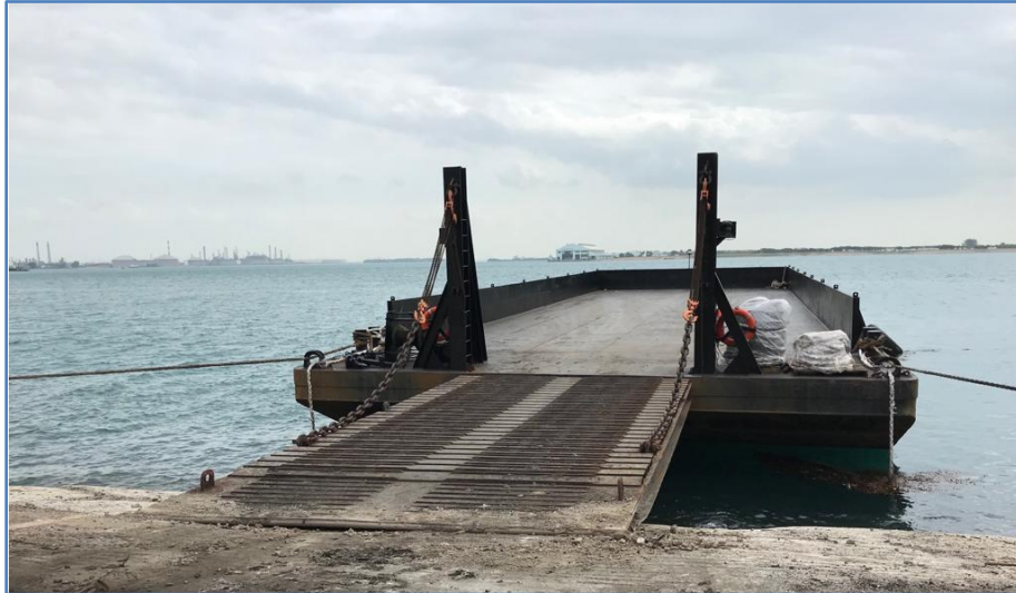
Figure 22 – Bow ramp door lowered at berth, sample photo for reference (Source: TSIB)
