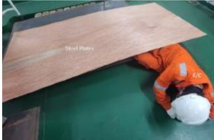
Figure 4 – Re-enactment of the EC's position when pinned down on the floor by the fallen steel plates ( Source: the Company )
