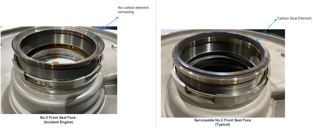
Figure A1: Seal face on event engine with missing carbon seal (left) compared to typical seal face with intact carbon seal (right)
