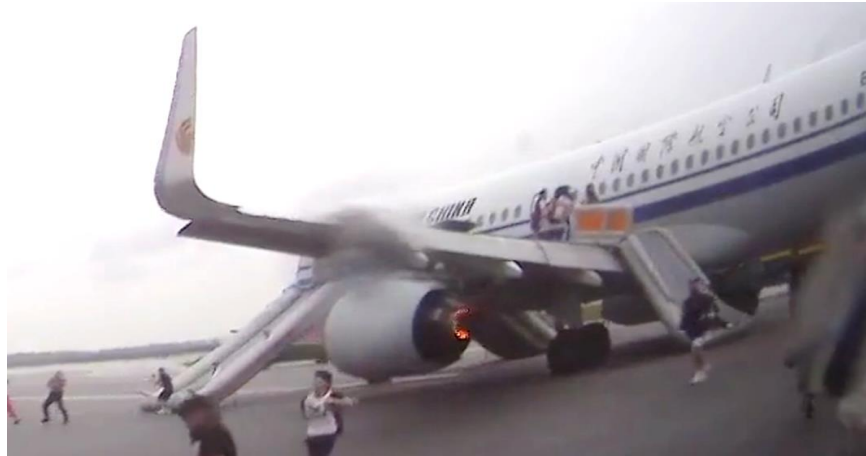
Figure 1: Fire at the tailpipe of left engine (Footage from T33's dashcam)
