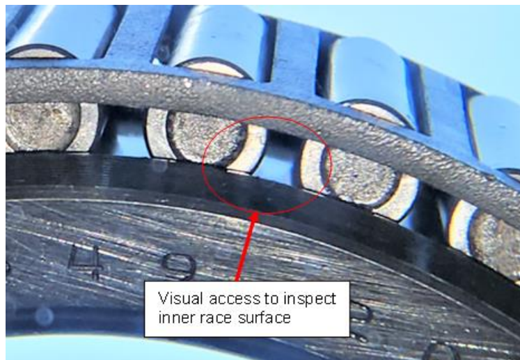
Figure 7: Inspection of inner race surfaces
