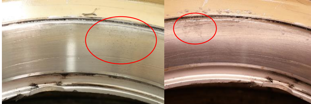
Figure B10: Outboard bearing cup surface with light traces of corrosion
