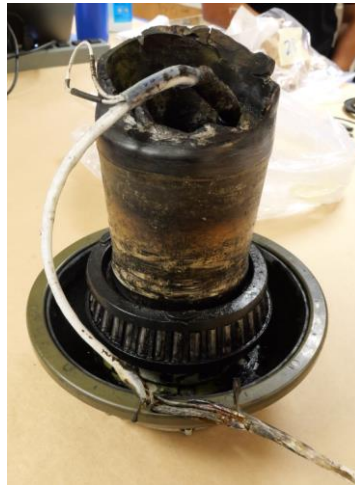
Figure 4: Outboard portion of the sheared off left axle with severed wire bundle
