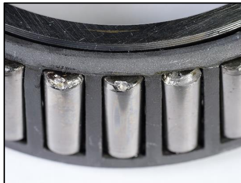
Figure B2: Damage on outboard bearing rollers
