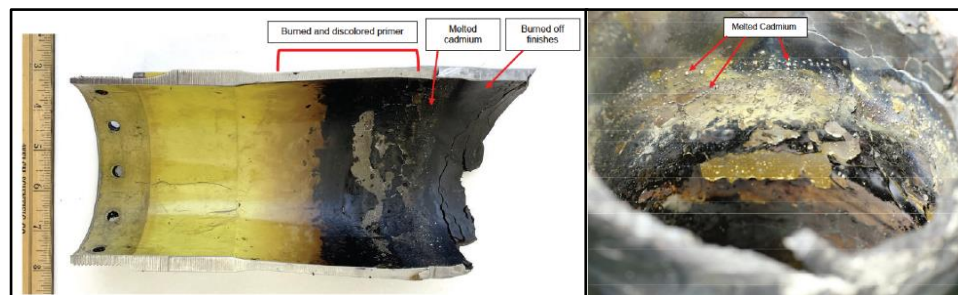
Figure B7: Discoloured and burnt primer with traces of melted cadmium
