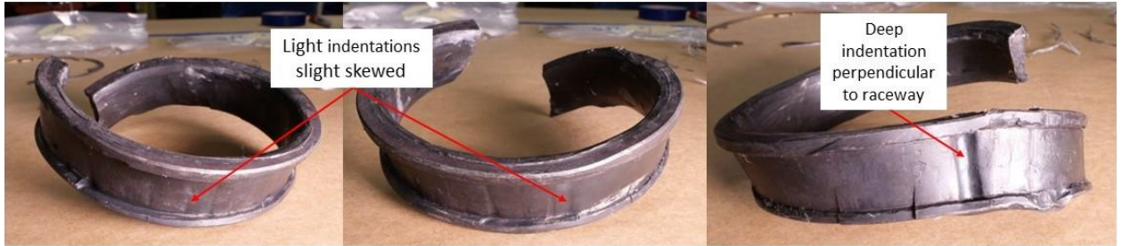
Figure 6: Several light skewed indentations and a deep indentation on inboard bearing cone
